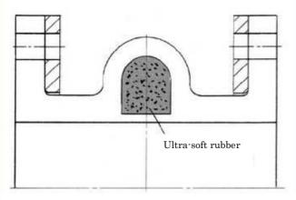
%In case of severe use conditions such as high temperature, high pressure or large amount of displacement, a metal ring may be used to reinforce a flange part, and the length of the surface of some sizes becomes slightly longer.
