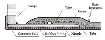
Inner part of the coupling is rubber lined to reduce an abrasion of the nipple by fluid. Fixed flange and loose flange are provided.
